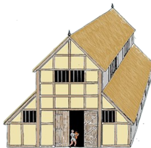
30: building F4 if posts supported the aisle of a timber-framed structure (Millum 2017)
