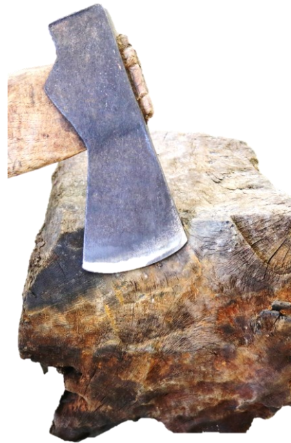
Fig. 8. Axe cut end of SF.5.79 showing axe marks and 75mm axe head
