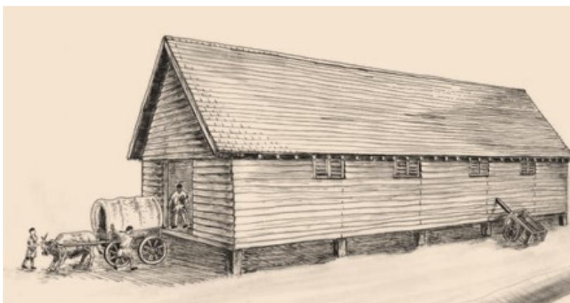
4.14: An interpretation of the 13-post building if made of plank walls with a shingle roof
