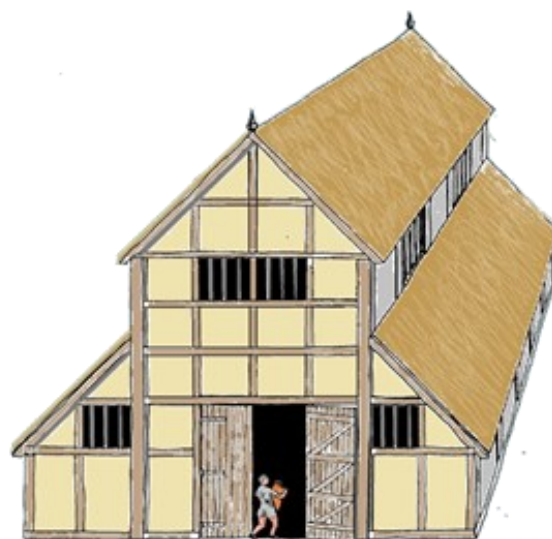
4.15: The building if the posts were a supporting aisle of a timber-framed wattle and daub structure with a thatch roof
